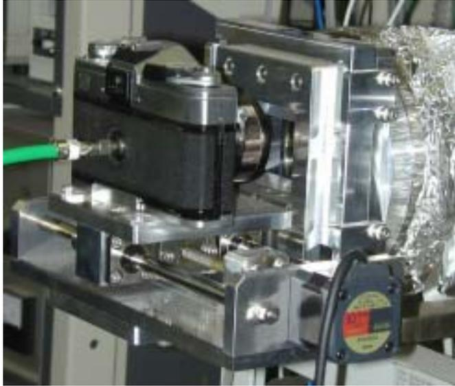
We observed the optical emission from the plasma with an equipment shown in this photograph. There is a quartz viewport of 7 times 5 centimeters, and the sputter chamber is located at the right side of this photo.
